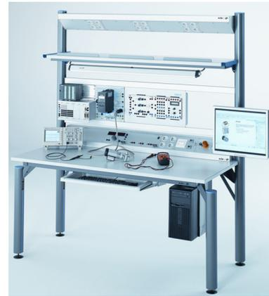
The modular design of the training system allows for applications which go above and beyond the limitations of the individual training packages. For example, PLC actuation of pneumatic, hydraulic and electric drives is possible.
