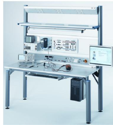
The modular design of the training system allows for applications which go above and beyond the limitations of the individual packages, such as, for example, PLC actuation of pneumatic, hydraulic and electric drives is possible.
