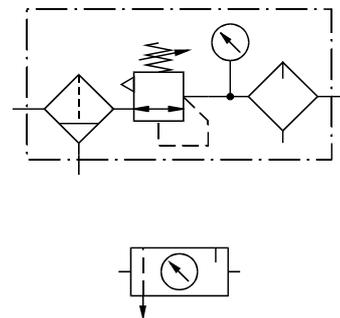
The compressed air filter has the job of removing all contaminants from the compressed air flowing through it as well as water which has already condensed. The compressed air enters the filter bowl through guide slots. Liquid particles and larger particles of dirt are separated centrifugally collecting in the lower part of the filter bowl. The collected condensate must be drained before the level exceeds the maximum condensate mark, as it will otherwise be re-entrained in the air stream.
