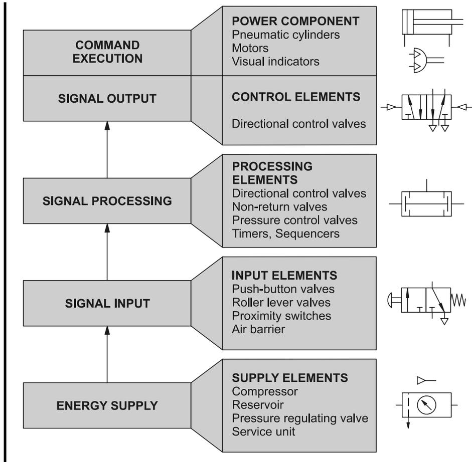
A directional control valve can be used as an input, processing or control element. The distinguishing feature for the allocation of the individual components to the respective groups of elements is the configuration within a pneumatic system.
